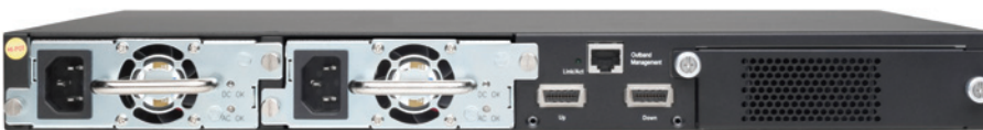
Figure 3. Brocade FCX-S switch models feature internal redundant hot-swappable power supplies and a swappable fan assembly, in addition to dedicated stacking ports and a rear-facing out-of-band management port.
